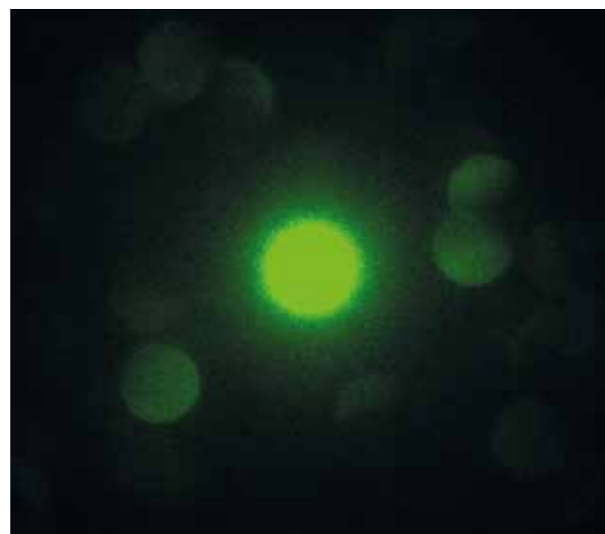
Precessed CBED pattern from a mapping experiment
