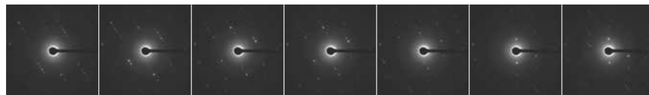
Electron Diffraction tomographic tilt series of Carbamazepine and reconstructed structure
