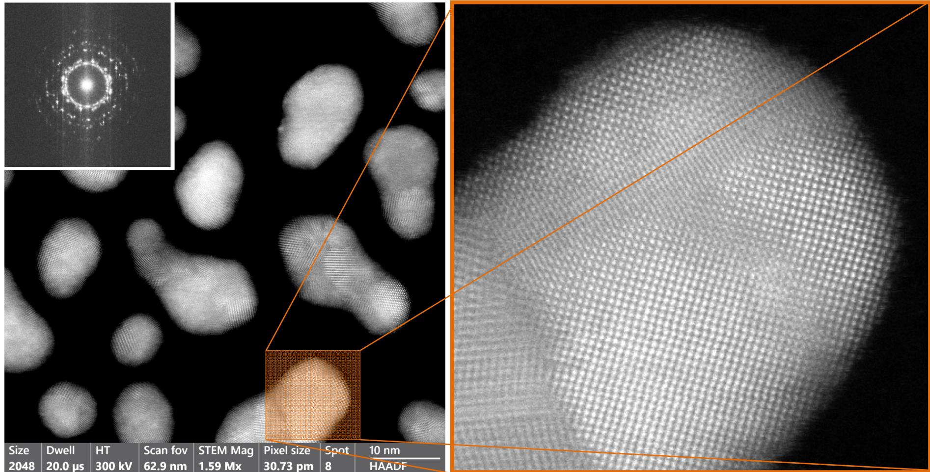
HAADF STEM image of gold grains on amorphous carbon at cryo temperature (< -170°C). It was acquired with ThermoFisher Spectra Ultra STEM using Simple Origin cryogenic inert gas / vacuum transfer holder Model 206. Courtesy of Dr. Nestor J. Zaluzec, Argonne Natl. Lab, USA
