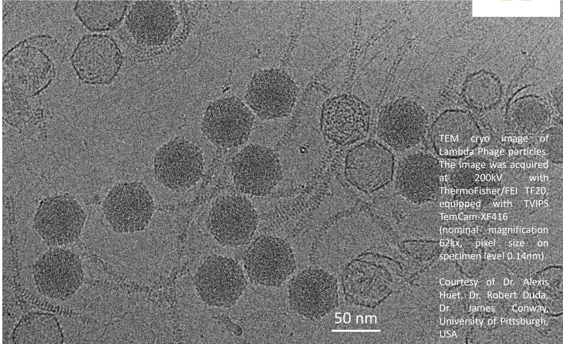
TEM cryo image of Lambda Phage particles. The image was acquired at 200kV with ThermoFisher/FEI TF20, equipped with TVIPS TemCam-XF416 (nominal magnification 62kx, pixel size on specimen level 0.14nm).
